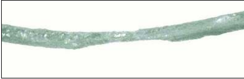
Figure 11. Outer wire of outer strand showing abrasion at the contact points as well as corrosion.
