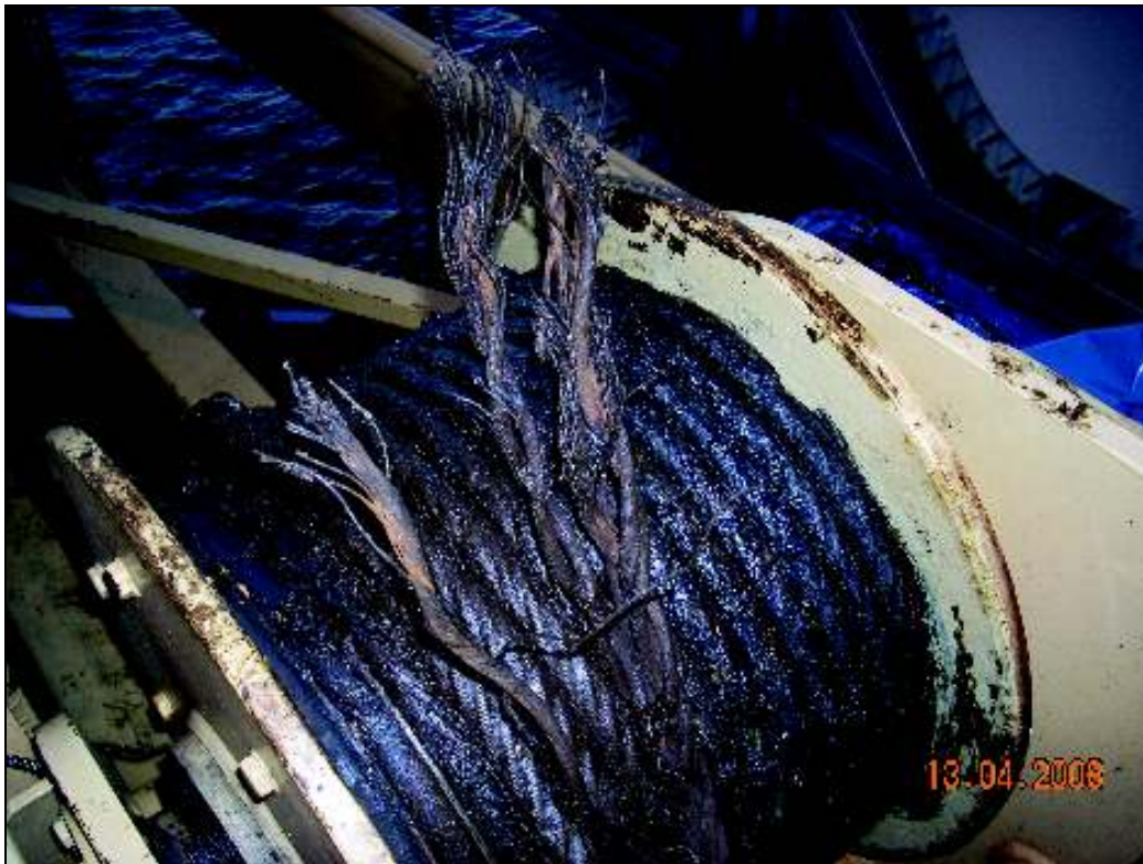
Figure 5. View of failed hoist wire at winch drum showing level of greasing present on wire during normal operation. Corrosion product is also visible on the de-stranded wires at the point of break.
